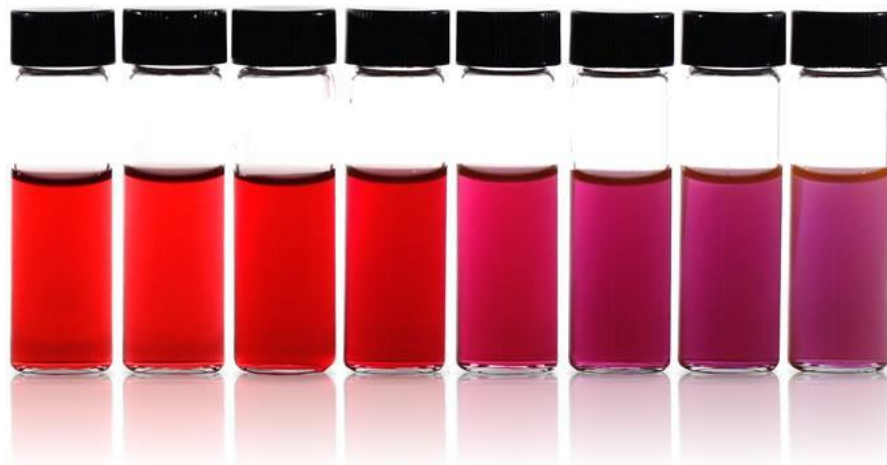
Figure 1.1: Colloidal suspensions of gold nanoparticles. As the nanoparticle diameter is increased from 5nm to 100nm, the scattered light from the suspension changes from red to purple. This is because the surface plasmon resonant wavelength increases with increasing nanoparticle size. Thus, for the smallest nanoparticles, blue wavelengths are absorbed from white light, while for the largest nanoparticles, red wavelengths are absorbed from white light. Image from nanoComposix.
