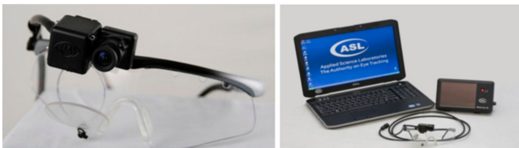
Figure 2. ASL mobile eye XG glasses on the left, complete equipment with data transmit unit (DTU) on the right.
