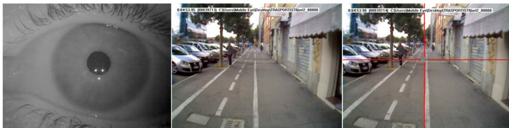
Figure 3. Superimposition of the eye tracking output to the cyclist's visual scene.
