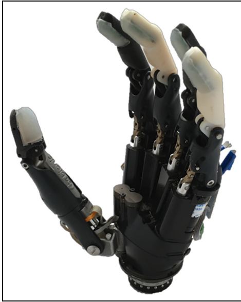
Figure 1. Modified Bebionic hand (RSL Steeper, Inc.) with multi-modal PCF tactile sensors at each finger.
