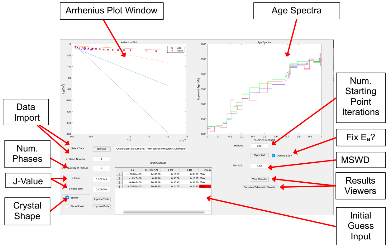
Figure 7: Labeled image of OPTIMuM's GUI with data (red) from Swindle et. al. (2009) sample LAP 031308A, thermal model (green), and ^{40}\text{Ar} distribution model (blue). See text for full model results.
