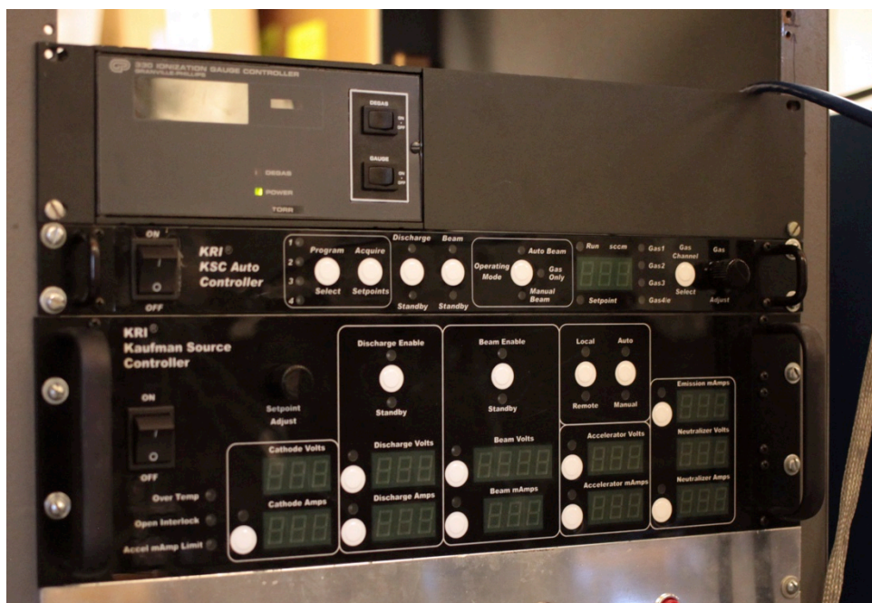
Figure 2.5: Ion gauge controller, flow controller, ion source controller (from top to bottom)
