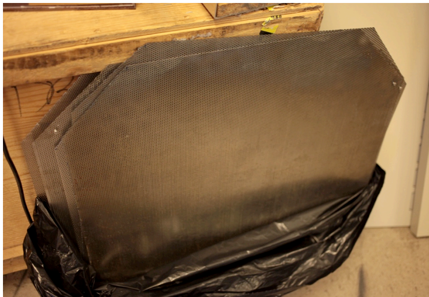
Figure 2.16: Perforated steel attenuators
