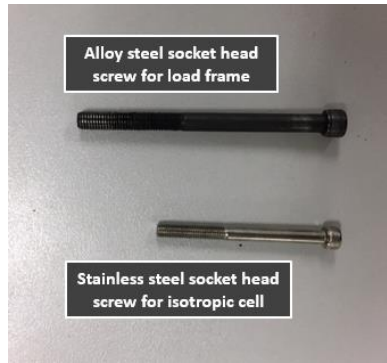
Figure 5.14: Socket head screws for load frame (above) and for isotropic cell (below)
