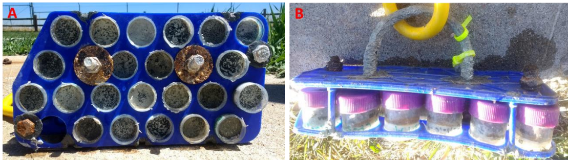
Figure 3-4. Example views of approximate volume and mass casted mortar samples installed in polypropylene racks secured with epoxy coated-stainless steel bolts and rods. A) bottom view. B) Front view.
