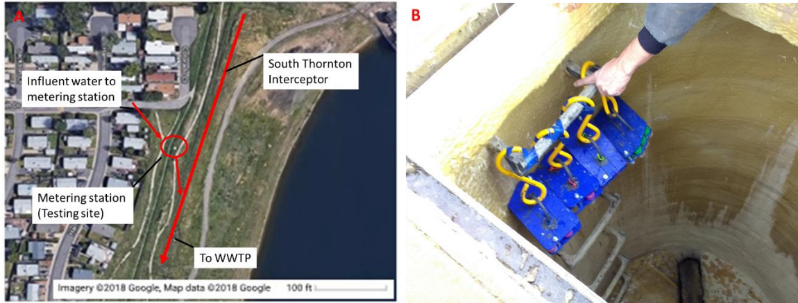
Figure 3-5. A) Map from the testing location. Red arrows indicate flow direction. The red circle shows the reclaimed metering station (LAT, LONG: 39.851046, -104.943181) used for accelerated corrosion studies. B) Photograph of the polypropylene racks installation in the manhole steps.
