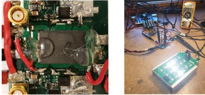
Figure 3.8: Planar integrated magnetics ZVS Ćuk converter prototype, and a test bench with LED's as the load.
