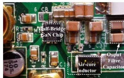
Figure 6.5: Photograph of the 100 MHz synchronous buck converter prototype using the GaN chip in the 20-pin 4mm × 4mm QFN package and 47 nH air-core inductor.
