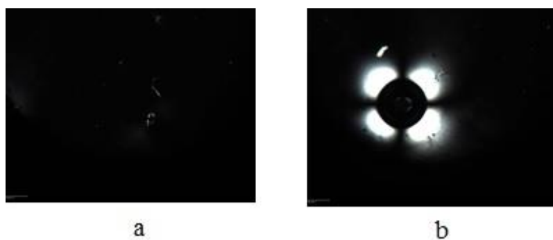
Figure 6.9. PLM images for (a) bulk, unpolymersized sample of air-free specimen, and (b) air-free polymerized film (mag = 50x). The bright regimes in PLM (b) appear to be defects. The majority of the sample was black. Because there were multiple defect sites, sample was not adequate to attempt membrane fabrication.
