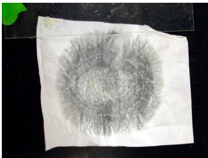
Figure 4.6. LLC/v-EPDM/H 2 O blend that has been fully infused into a Solupor® support membrane. The sample shows some inhomogeneity from visual inspection, as well as no discernible LLC phase via XRD characterization.
