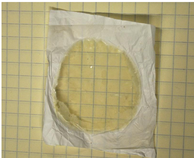
Figure 3.S9. Picture of a supported cross-linked Q I -phase membrane of 4a . Scale: Each grid division is 0.25 of an inch. The polymerized Q I -phase of 4a infused into the Solupor support is visually transparent, while the surrounding pristine Solupor support material is not.
