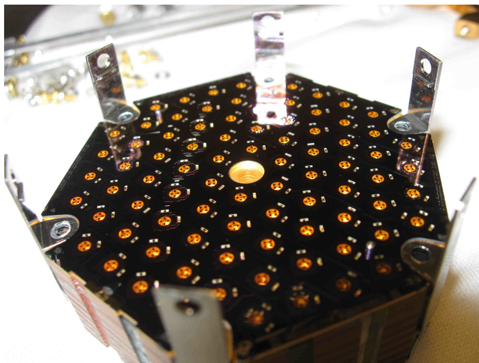
Figure 3.3: (Top) Schematic of one SPTpol 150 GHz pixel. Areas with white hashing are regions where the silicon substrate has been etched away leaving released silicon nitride. (Bottom) One of the seven SPTpol 150 GHz detector arrays during module assembly, before installing the BS wafer. The array is 2.3 inches across.
