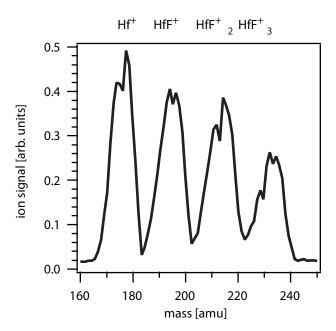
FIG. 5: Mass spectrometry. Operating the rf (Paul) trap as a quadrupole mass filter gives mass-dependent trapping potentials such that  $\mathrm{Hf}^+$  ( $M=180~\mathrm{amu}$ ),  $\mathrm{HfF}^+$  ( $M=199~\mathrm{amu}$ ),  $\mathrm{HfF}_2^+$  ( $M=218~\mathrm{amu}$ ), and  $\mathrm{HfF}_3^+$  ( $M=237~\mathrm{amu}$ ) can be separately trapped and detected. The ion detector signal is a non-linear function of ion number, but a level of 0.4 corresponds to  $\sim 100,000$  ions.
