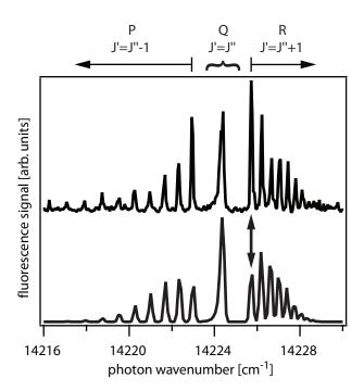
FIG. 4: Laser induced fluorescence (LIF) spectroscopy. The top trace is experimental data for a newly detected neutral HfF transition:  $[14.2] |\Omega| = 3/2 |v' = v'', J'\rangle \leftarrow X^2 \Delta_{3/2} |v'', J''\rangle$ . The transition highlighted with a vertical arrow originates from the rotational ground state. The bottom trace is a theoretical prediction assuming a rotational temperature of 5 K. The traces are offset vertically for clarity.
