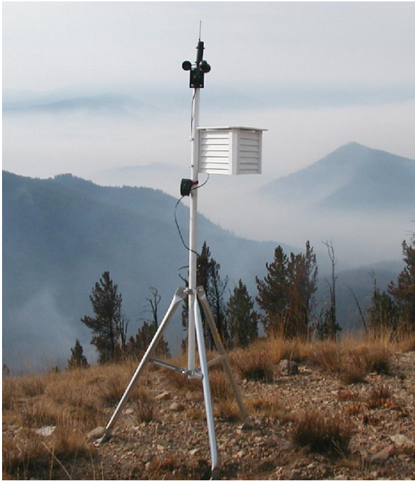
(a) An enclosure we built for our sensor nodes. The open bottom, vented ceiling, and slotted walls allowed the sensors to accurately record conditions.
