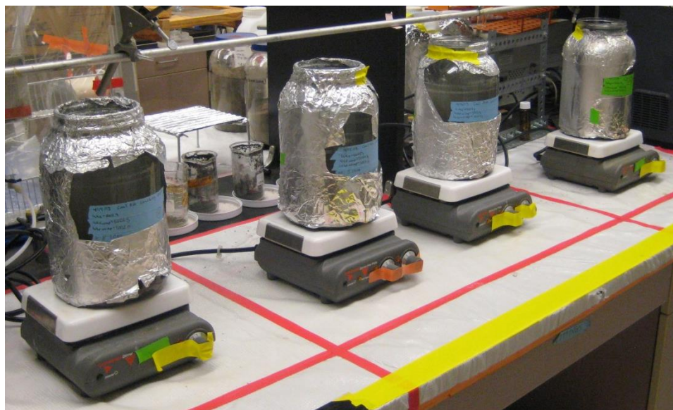
Figure 3.2. Experimental setup to release elements from coal ash under oxic condition. The three coal ash reactors are colored blue, and the control reactor is colored green.
