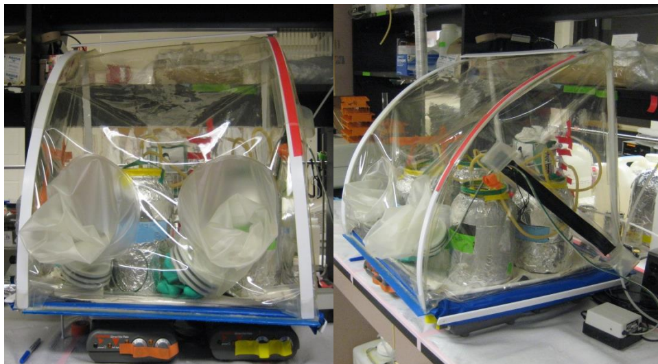
Figure 3.3. Experimental setup to release elements from coal ash under anoxic condition. The three coal ash reactors are colored blue, and the control reactor is colored green.
