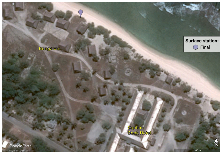
Figure 2. Aerial view of the Captain Cook Hotel property on Kiritimati, including the CXENRR site (upper left). The final location of the surface meteorology instruments is at the base of the pin symbol, north-northeast of the bungalow that housed staff and the Vaisala DigiCORA sounding system. The concrete pad where the helium tanks were stored and from which balloons were launched runs northwest to southeast, ending just north of the bungalow. The main hotel building used for Internet access is southeast of the CXENRR site.
