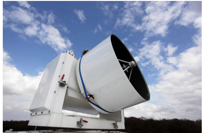
Figure 1. Scanning Ka-band Doppler cloud radar JOYRAD-35 (JOYRAD-35 system) installed at the JOYCE site, Jülich, Germany. Technical specifications of the radar are provided in Table 2.
