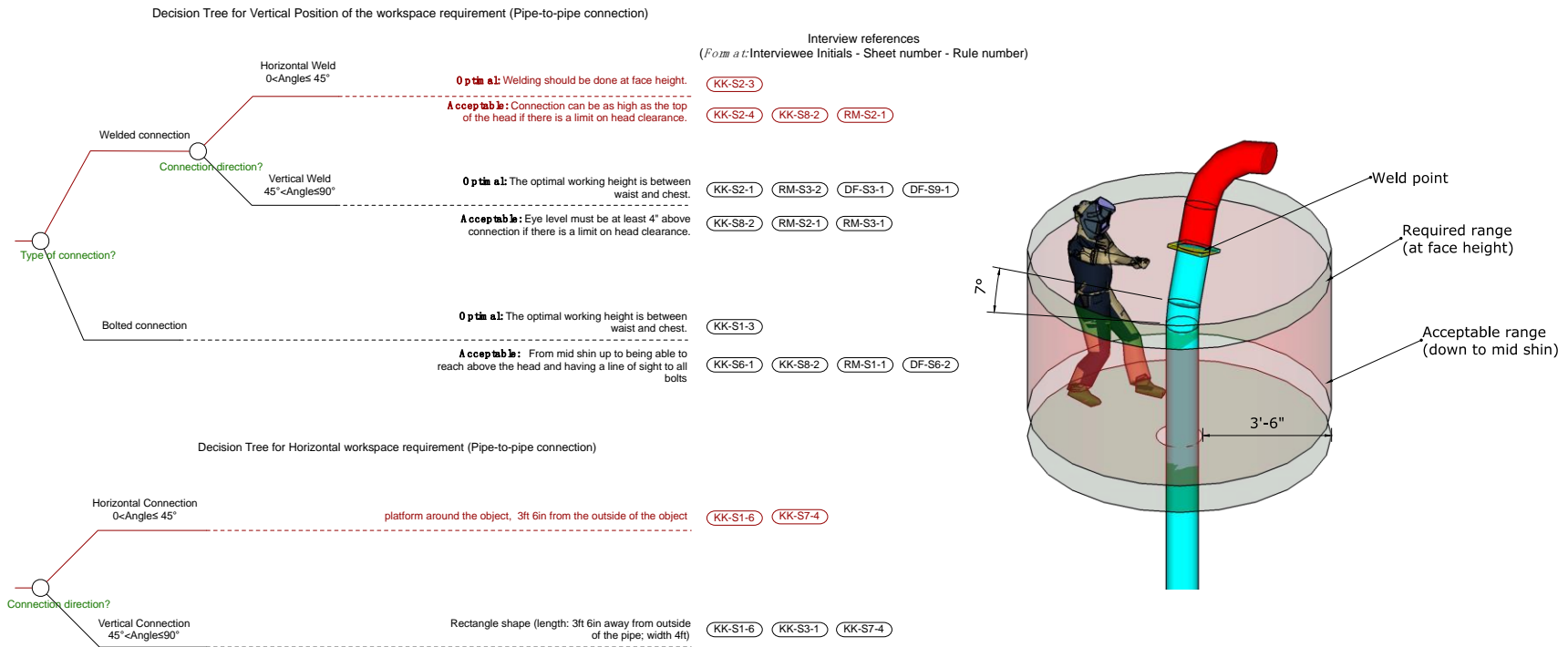
FIGURE 8: Decision tree for a pipe-to-pipe connection.
