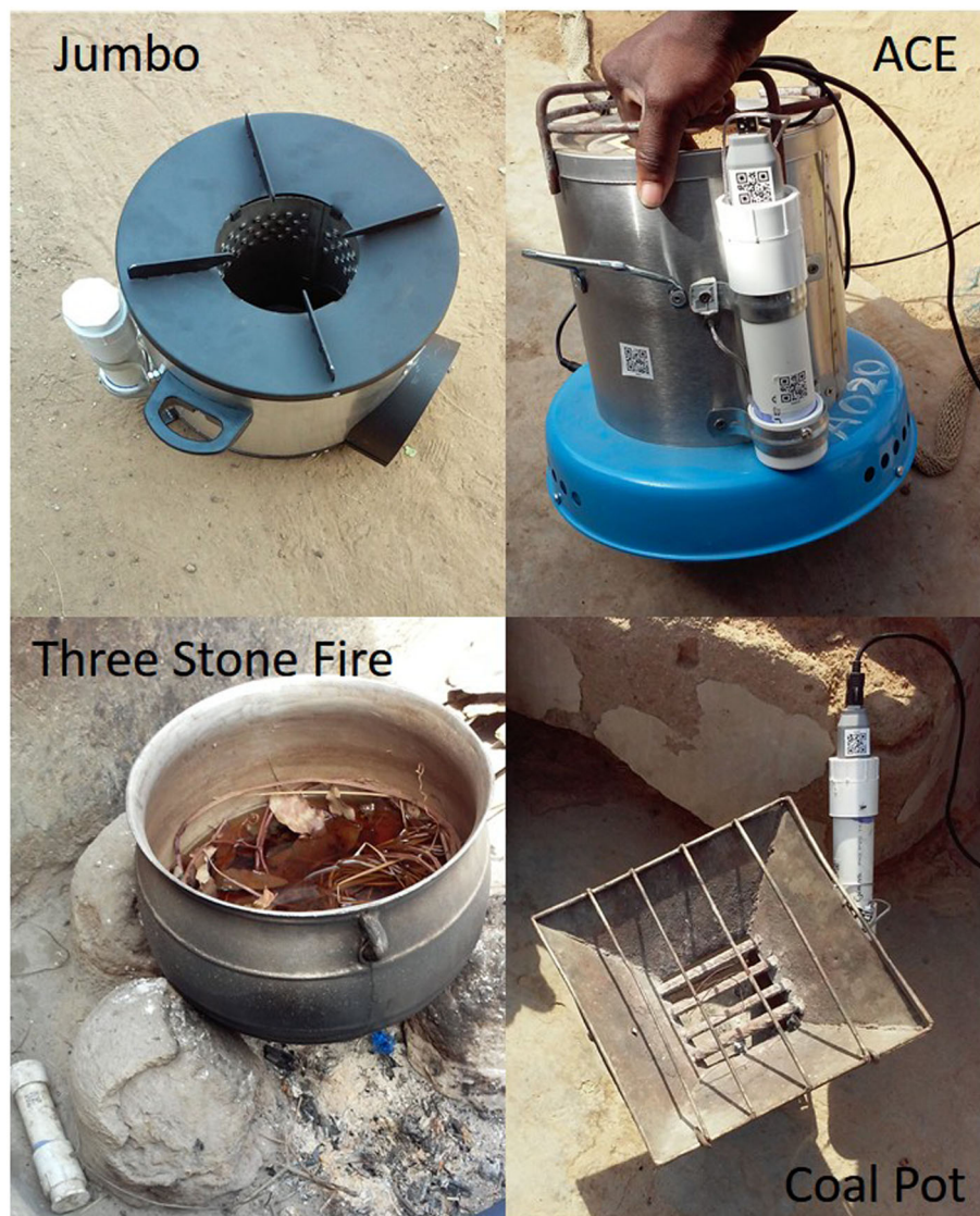
Fig. 5 Placement of stove use monitors (SUMs) on improved stoves (Jumbo and ACE) and traditional stoves (Three Stone Fire and Coal Pot). Images source: study authors
