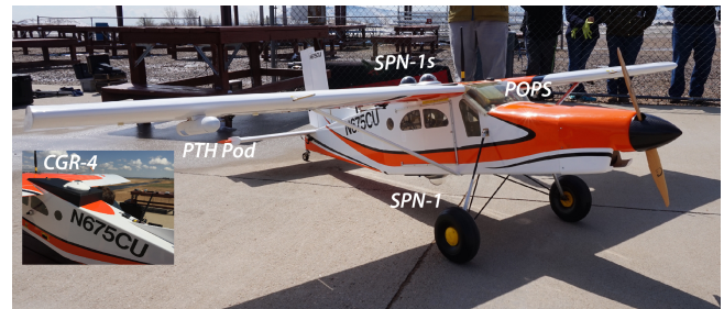
Figure 1. The RECUV Pilatus UAS shown with PTH module (white pod on starboard wing), POPS aerosol spectrometer (gold box in windshield), and three SPN1 pyranometers (two sensors on roof and one sensor on belly). The inset shows the aircraft with the upward-looking CGR4 mounted.
