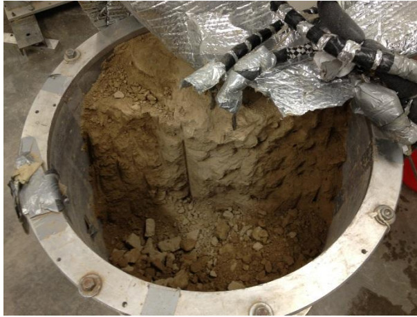
Figure 7.10 Post-test profile section of the unsaturated silt layer showing the drying zone within the heat exchanger array in Test 1
