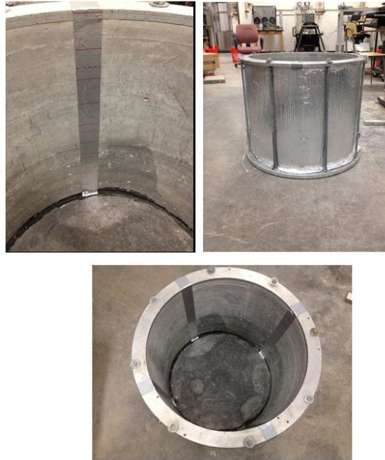
Figure 6.1 Experimental container with sensor level markings
