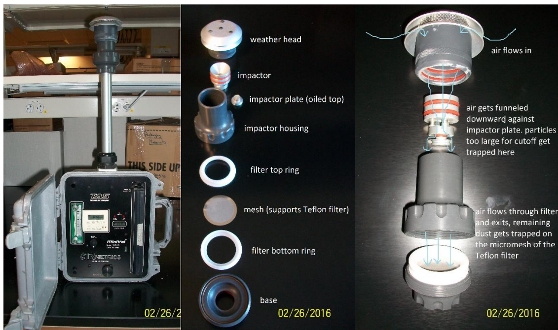
Figure V: MiniVol Filter Assembly (PM 2.5)
