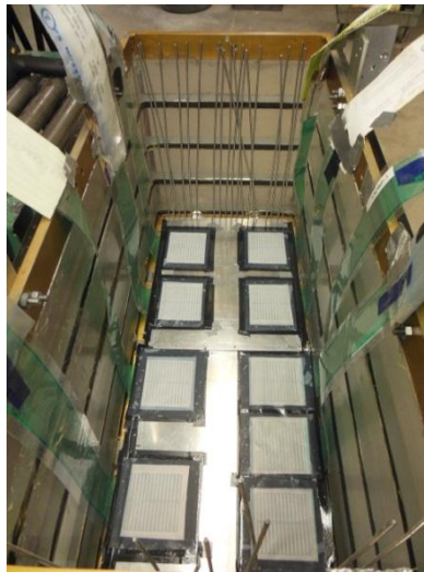
Figure 5.4. Polished aluminum plates with attached tactile pressures sensors and two Teflon sheets placed at the bottom of a centrifuge container prior to sand pluviation.
