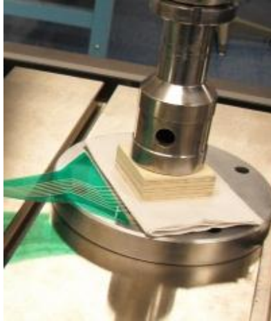
Figure 4.18. Steel plate – pressure sensor – paper towel – wooden block – loading machine interface
