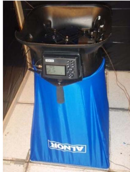
Figure 3–29: Balometer Capture Hood
