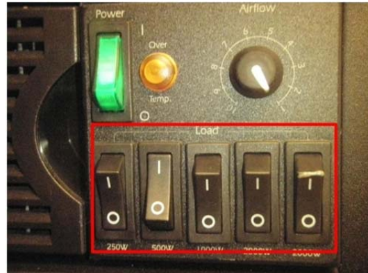
Figure 3–21: Heating Element Control Switches
