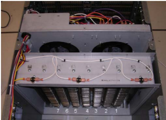
Figure 3–20: Server Simulator Heating Elements 21
