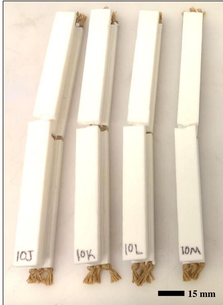
Figure 22. Flexural composite specimens post-break.
