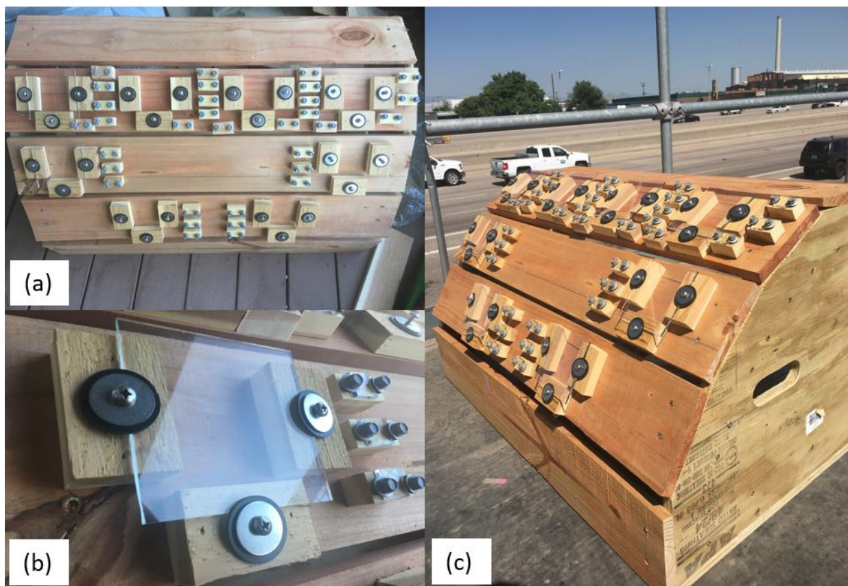
Figure S1. The wooden frame after installing all the stands for both the small and large glass samples (a); The large and small glass samples after fixing them on the stands (b); The whole wooden frame after placing it on the site (I-25 Globeville) (c).
