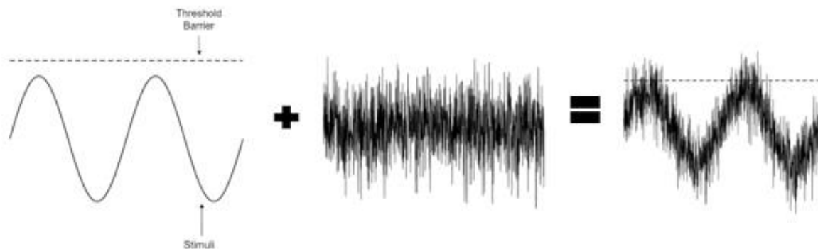
Figure 1. Visual representation of the non-dynamical model of SR. The threshold barrier represents the magnitude where signal perception is achieved. A nonlinear signal with a magnitude lower than this barrier may never be recognized. Adding noise to the signal allows information to cross this barrier.
