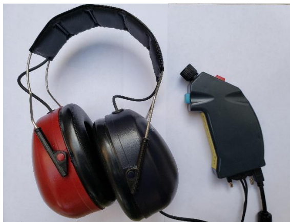
Figure 6: Visual image of testing equipment. The red cuff is placed on the right ear, blue on the left. Subjects hold the CHA during the exam and press down the blue button when they hear tones.
