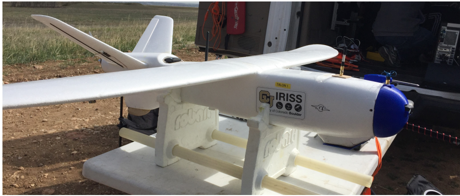
Figure 5.2: A picture of the Talon UA setup for an RF localization mission with multiple antennas including a 900MHz telemetry radio, 2.4GHz C2 link, and a 5.8GHz binary direction finder setup
