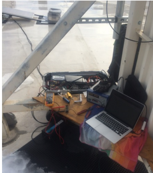
Figure 3.10: The setup for the onsite calibration of the station current monitors. Note the power supply and power resistor providing a variable current flow for measurement purposes.
