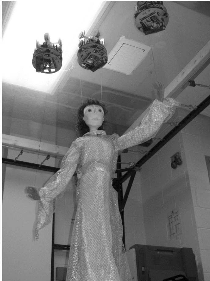
Figure 7. Three robotic controllers operate a traditional wooden marionette suspended from a plastic ceiling that covers the stage. The robots each control two puppet strings and collaborate with each other to perform the motions of a puppeteer and generate marionette motion.
