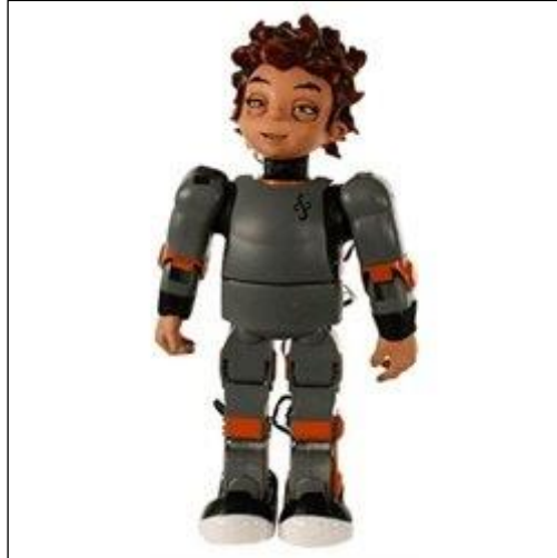
Figure 4. RoboKind (developed by Hanson Robotics) is an autonomous walking robot that is capable of expressive facial gestures based on interactions with human users.
