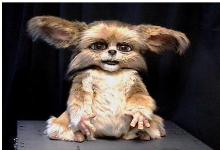
Figure 11. Despite its animal-like appearance, Leonardo is considered a humanoid robotic because it is designed for traditional social interactions based on human communication strategies.
