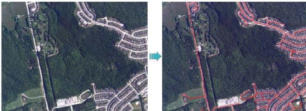
Figure 2.3 An example of an automatic detection method of road network extraction from areal imagery. Extracted roads are displayed in red ( http://gis.incogna.com/?p=technology#Road , accessed June 2013)
