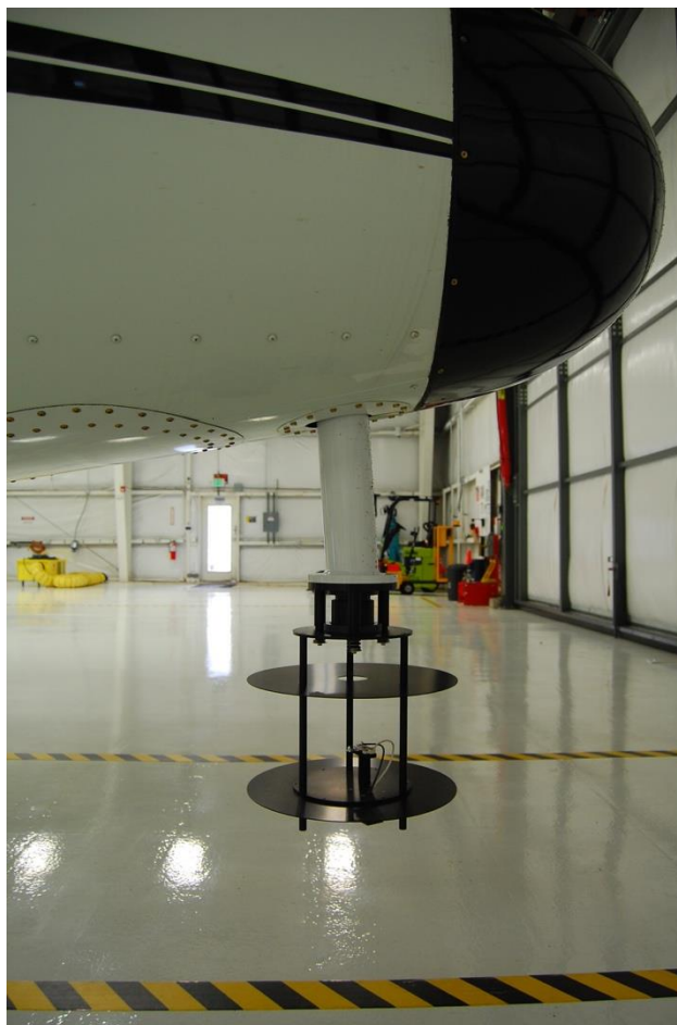
Figure 2.8: Universal field calibrator installed on the SSIM nadir light collector. Calibrations were made in the hangar while the SSIM was installed on the NEON Twin Otter. An opaque two-layered black shroud (not pictured) covers the light collector and calibrator when in use.
