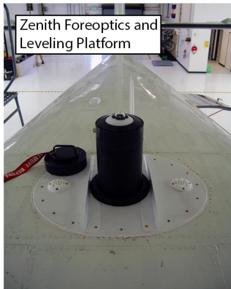
Figure 2.3: Photographs showing the SSIM foreoptics installed on the NEON Twin Otter. The zenith pointing light collector includes the leveling platform and is located mid-fuselage. The nadir light collector is fixed and mounted below the aircraft's nose.
