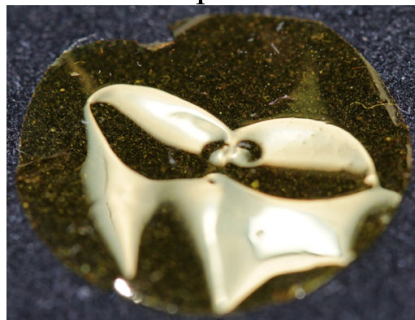
Fig. B.2 An example of a +2 defect with fractal-like topography with two generations of 2-fold dimples. Exposed with two sided illumination.
