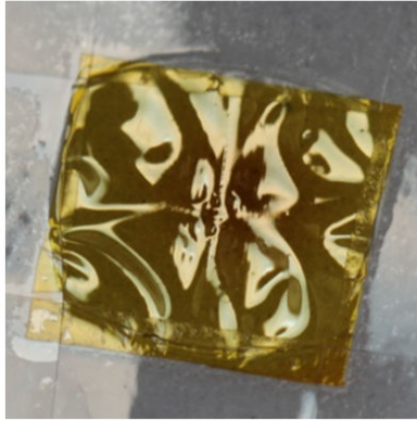
Fig. B.4 The deformation of -1 defect flattened and pulled taut.
