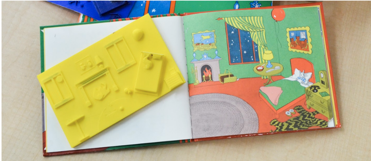
Figure 2.1. First 3D Printed Prototype of a picture from Goodnight Moon.
