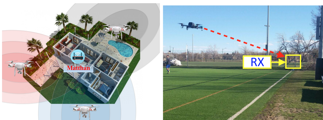
Figure 1.2: Matthan is a system to detect the presence of the drone by recognizing its body shifting and body vibration signature utilizing RF AP architecture. In particular, Matthan receiver captures the signal emitted from RF transmitters in the surrounding environment, and then analyzes the captured signals to detect the presence of drones to alert and protect their privacy. https://youtu.be/id2LxOsr_G8 .
