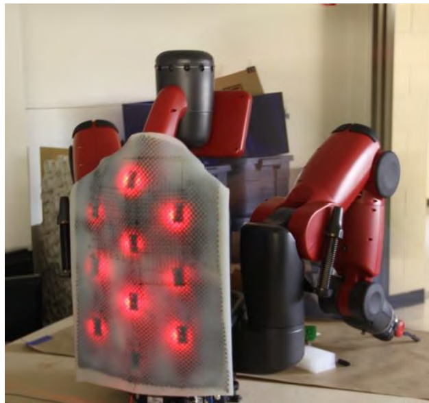
Figure 5.1: Amorphous skin mounted on the back of a Baxter robot.
