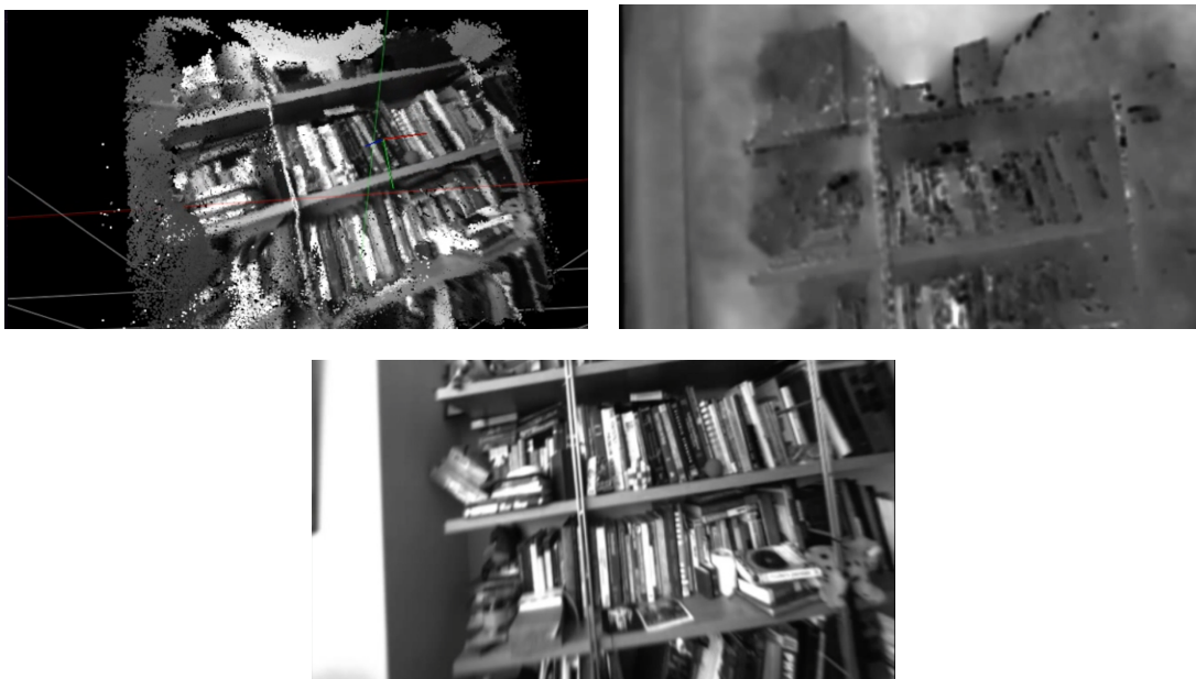
Figure 3.10: Point cloud (a), depth map (b), created from images (c) in a live data sequence using this algorithm. The scene depicts a camera scanning a bookshelf in a living room environment. High levels of fidelity, as those provided by volumetric approaches to 3D reconstruction, are important for robotic interaction in indoor environments.
