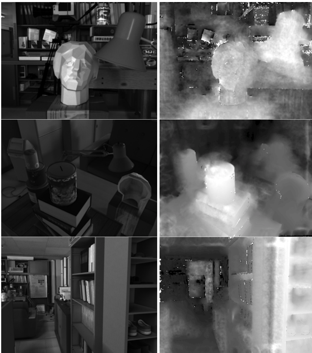
Figure 3.5: Images from the Tsukuba sequence with their corresponding depth maps generated with this approach. The first depth map is of inferior quality, as it corresponds to the start of the sequence where there is limited data and little movement.
