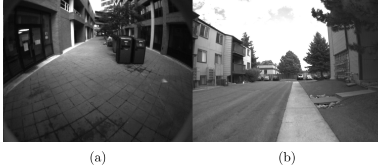
Figure 2.5: Comparison of images obtained from rig A (a) and rig B (b) as described in Section 4.3. Rig A is a mobile hand-held device with a wide-angle lens and a global shutter camera capturing at 30 fps and with 640 \times 480 resolution. Rig B is a custom hand-held device with a global shutter camera capturing at 30fps and with 1280 \times 960 resolution downsampled to 640 \times 480 . The picture quality and contrast of rig B is generally much better. Both rigs use a commercial grade MEMS IMUs: rig A sampled at 120Hz and rig B at 200Hz. Rig B features a much larger lens and higher quality camera.
