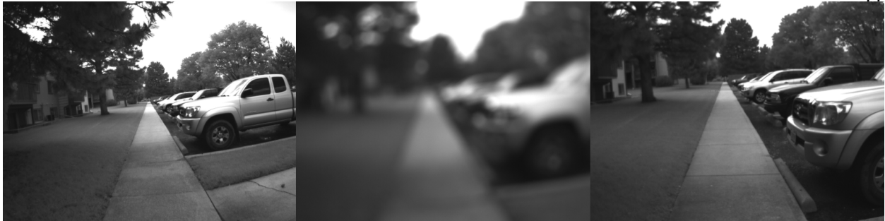
Figure 4.1: Online self-calibration during a zoom event in a \sim 200m sequence. The left image was captured just before the zoom event. The center image was captured during the zoom, where focus is temporarily lost, causing a total loss of feature tracks. The right image shows an image captured just after the zoom. This event is automatically discovered and new accurate camera intrinsics are re-estimated online in real-time.
