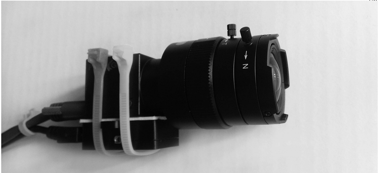
Figure 4.5: Experimental rig used to capture images (640x480 pixels at 30fps) and IMU data (at 200Hz). Consists of a USB camera attached to a USB commercial-grade IMU. The varifocal lens has adjustments for zoom and focus, with focal length variable between 4mm and 8mm.
