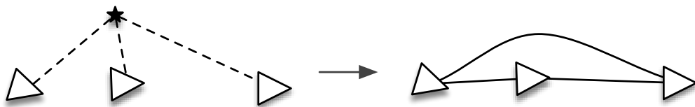
Figure 1.3: Once a landmark is marginalized, it induces new edges into the graphical model. These edges represent the influence of the landmark parameters on the remaining parameters of the optimization. As evident in the figure, the induced edges connect every pair of parameters which took part in a constraint with the original landmark parameters.
