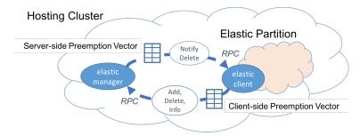
Figure 3.2: Experiment's elasticity facilitated by the exchange of preemption vectors.
