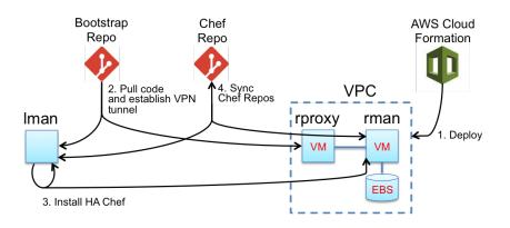
Figure 4.2: The deployment of the HA-enabled Chef with AWS components.
