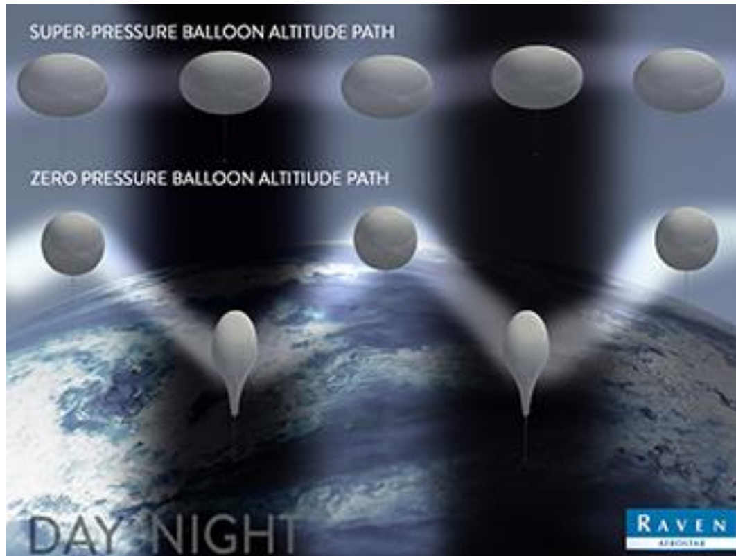
Figure 63. Super-pressure balloons altitude path at day and night [130].
