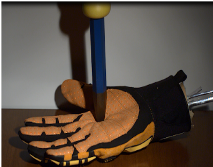
Figure 2 – Screen capture of a gloved hand being struck by a falling concrete chisel.
