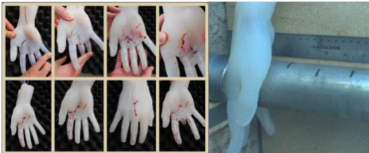
Figure 6 Artificial Hand Caught in the pipe and coupling pinch-point NIS
