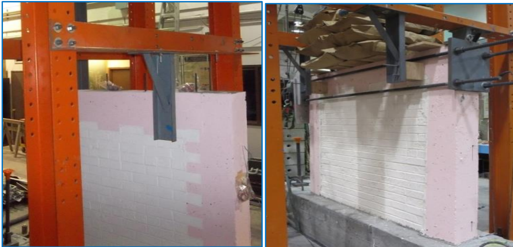
Figure 3-31. Lateral brace set up
