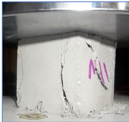
Figure 3-19. Mortar cube undergoes compression
