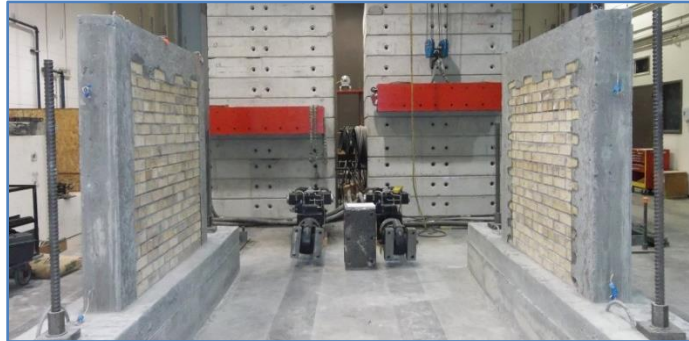
Figure 3-16. CM shear walls built in the SML
