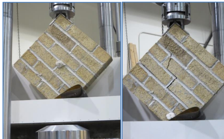
Figure 3-26. Diagonal Compressive Shear test
