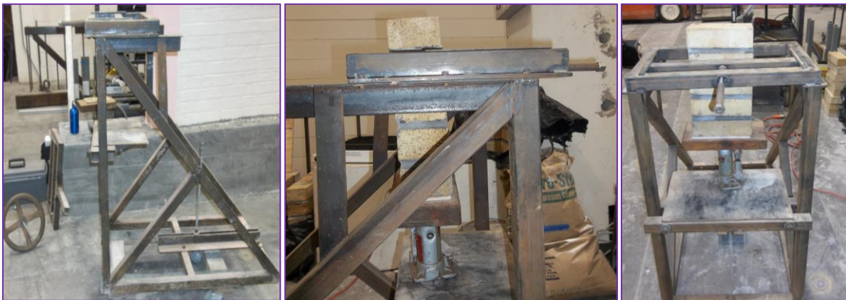
Figure 3-28. Bond wrench test
