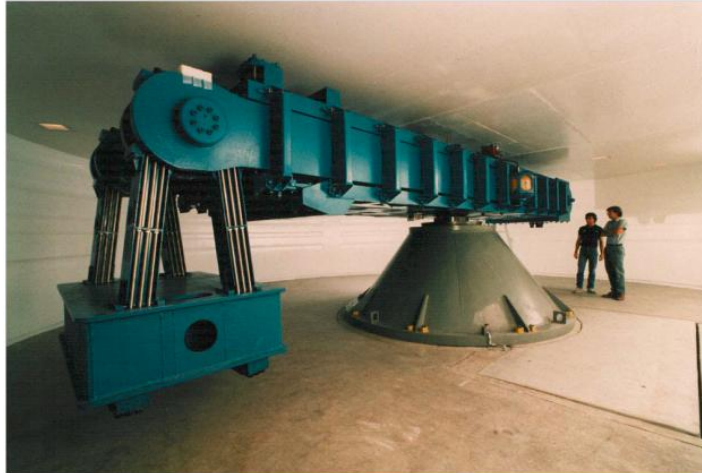
Figure 3-1. The 400-g ton centrifuge at the University of Colorado Boulder.
