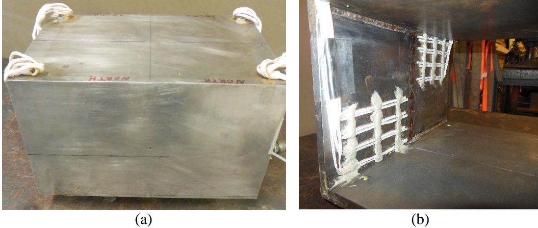
Figure 3-47. (a) Structure with no strain gages on the outside wall (b) installed Tokyo Sokki Kenkyujo strain gages on the inside wall of structure.
