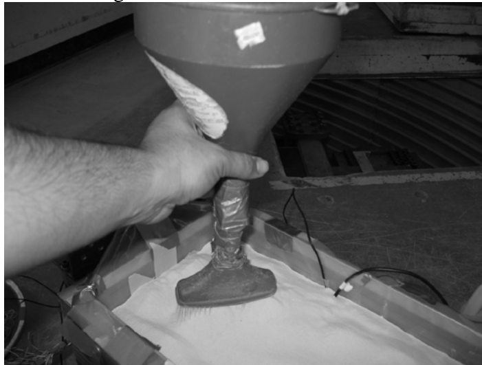
Figure 5-16. Sand layer preparation using dry pluviation
