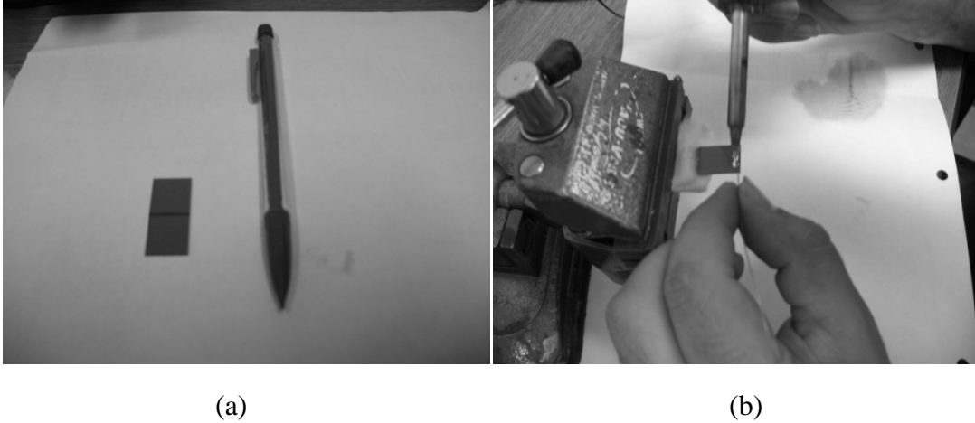
Figure 6-1. (a) T226-A4-303X type piezo-ceramic; (b) Soldering the coaxial cable
