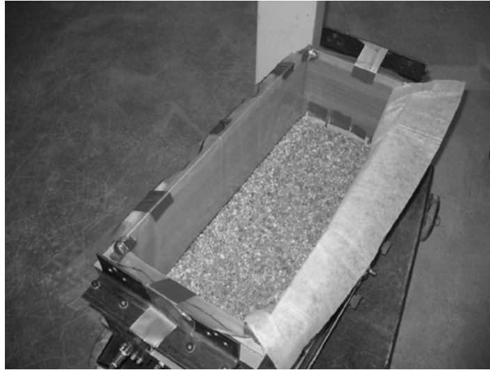
Figure 5-14. A layer of gravel served as a drainage layer
