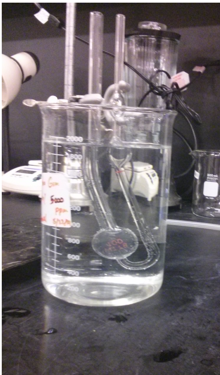
Figure D.1: Cannon-Fenske Routine Viscometer, size 100
