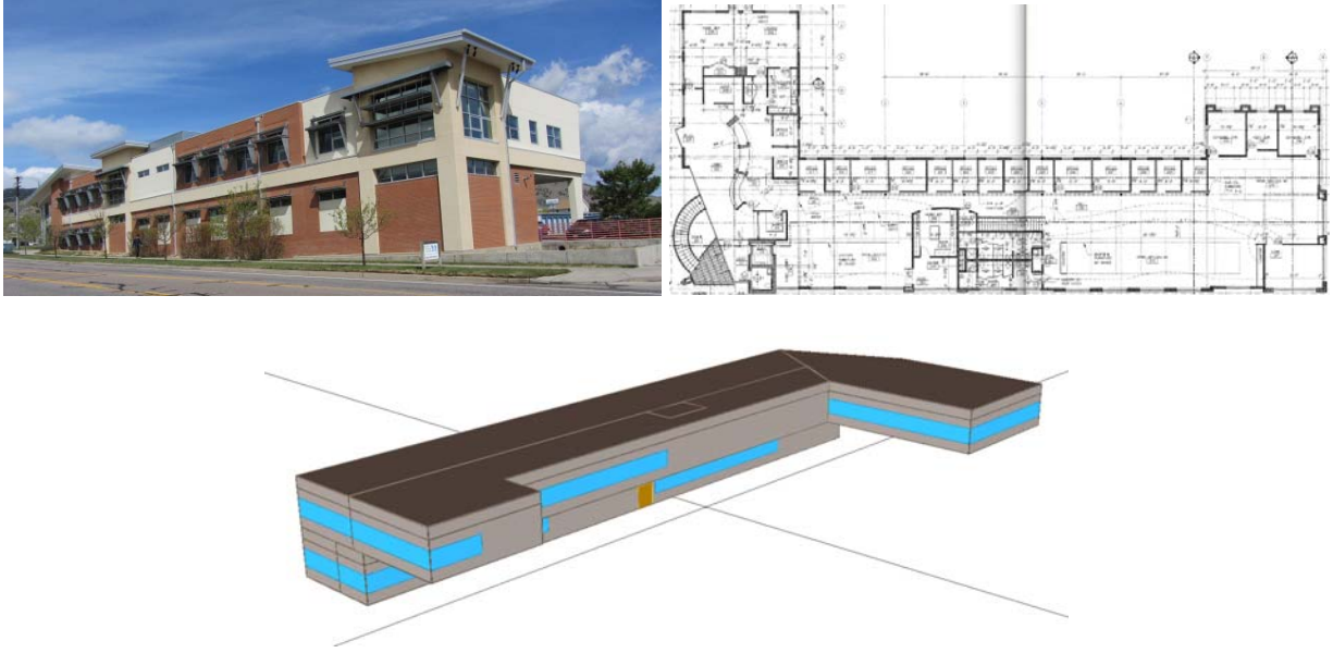
Figure 5-1. Exterior (top-left) of medium office building and its blueprint (top-right) and its eQUEST modeling screen (bottom)
