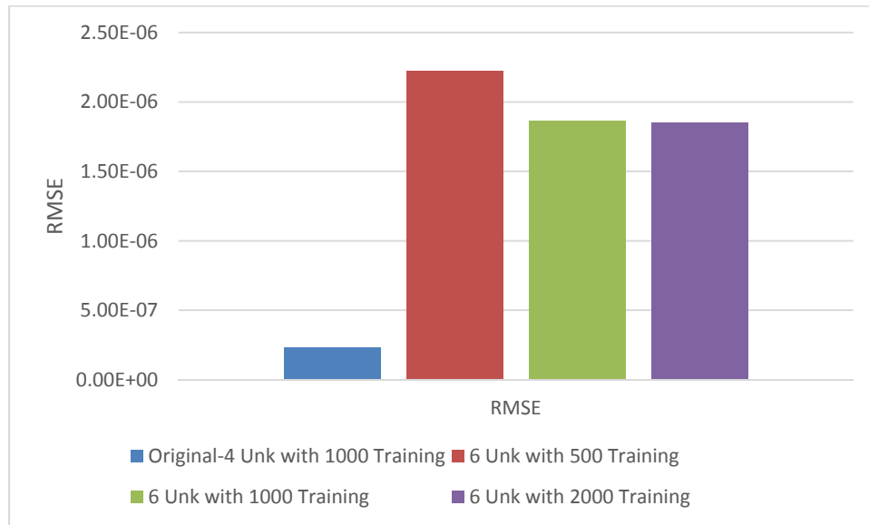
Figure 6-1. Comparison result of RMSE of 2 variables addition to an original emulator for residential building
