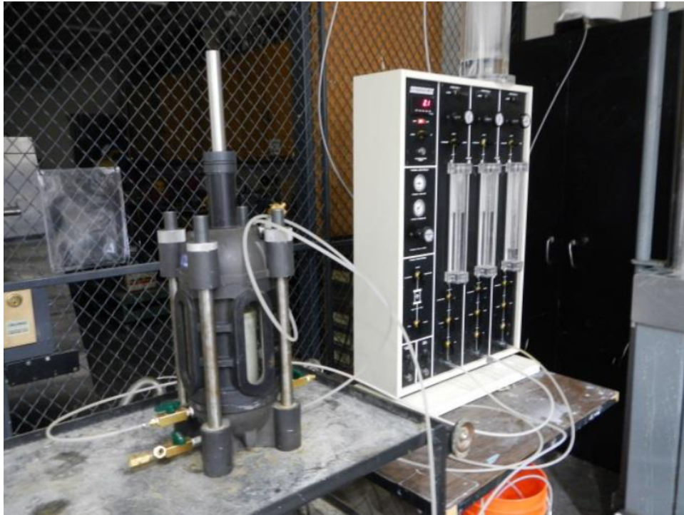
Figure 3.23: Triaxial Compression Test Apparatus from Svoboda (2013)
