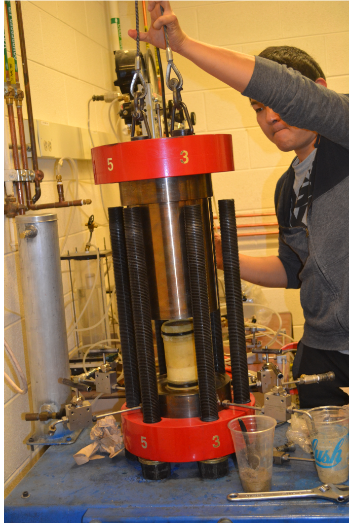
Figure 3.8: High Pressure Isotropic Compression Test Apparatus and Soil Sample
