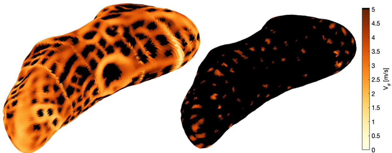
Figure 3.47: ( left ) Minimum and ( right ) maximum lift-off velocity across the J = 24 , sectored spherical harmonic model of Eros.
