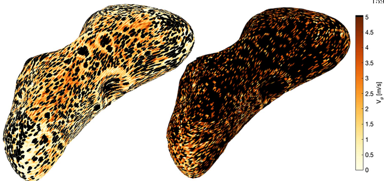
Figure 3.41: (left) Minimum and (right) maximum lift-off velocity across Eros's polyhedron model.
