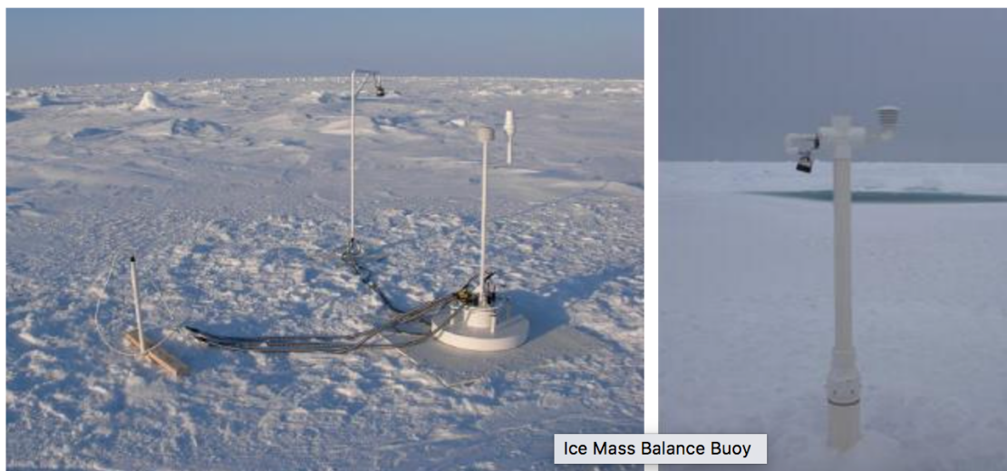
Figure 6.10: Two ice mass balance buoys installed in ice in the Arctic. Reproduced from http://imb.erd.c.dren.mil/index.htm
