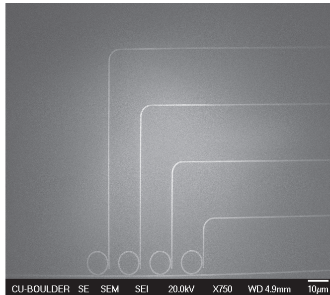
Figure 3.5: A SEM image of a wavelength-division multiplexer (WDM'er) that consists of four micro-ring resonators with 200-nm gaps and 450-nm waveguides. From left to right, the radii of the micro-rings are 4.975 \mu\text{m} , 4.995 \mu\text{m} , 5.015 \mu\text{m} and 5.035 \mu\text{m} , respectively.
