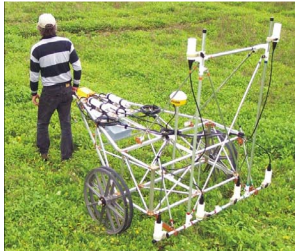
Figure A.11. Example of subsurface magnetic field measurement using an array of commercial atomic magnetometers. (Geometrics, Inc.)
