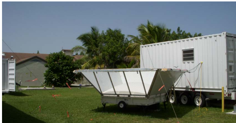
Figure 3.1. The MAPR 915 MHz spaced antenna wind profiler radar at the Center for Southeastern Tropical Advanced Remote Sensing (CSTARS) in Miami, FL.
