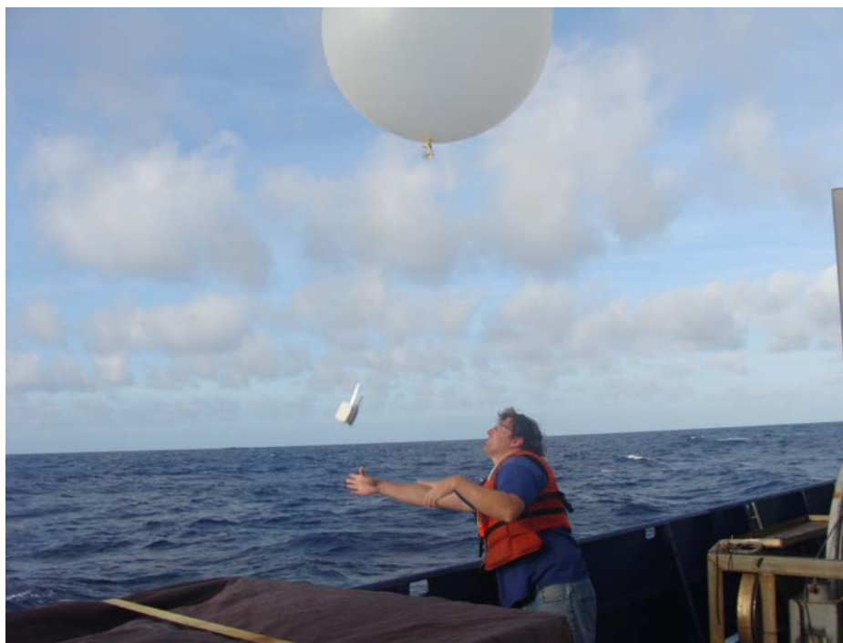
Figure 1.5. The author launching a radiosonde aboard the R/V Roger Revelle in the Indian Ocean as part of the DYNAMO project.
