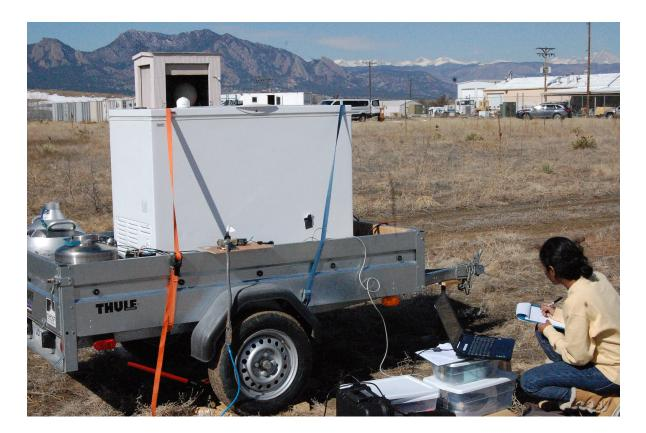
Figure 5.16: The calibration chamber housing the radiometer and calibration targets rests on a trailer as the radiosonde, seen in the background, is ready for launch [5] at the Marshall field.
